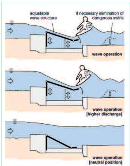
Figure 3. Adjustable wave structure (Dreamwave – concept)
