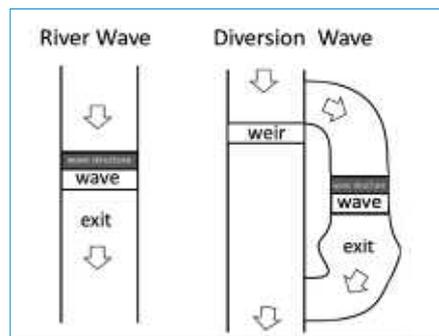
Figure 4. River wave concepts – different plan view situations
