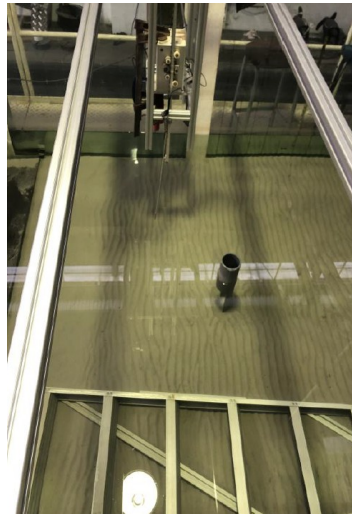
Figure 2. A view of the final bed form. The orifice plate was removed for measuring the bed levels under the OWC chamber.
