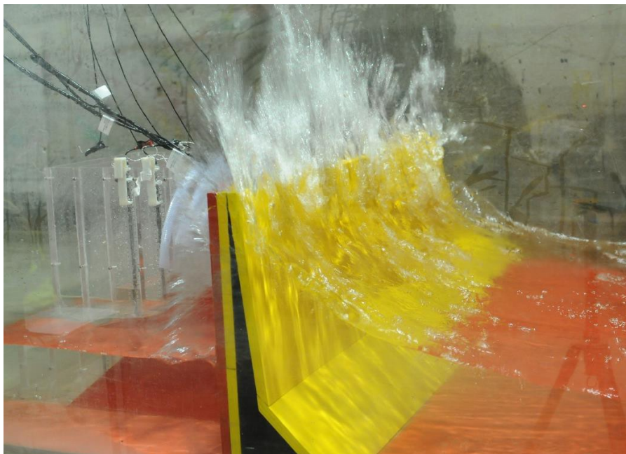
Figure 1. Airborne wave overtopping during flume tests and multi-chamber tank in the lee of the structure
