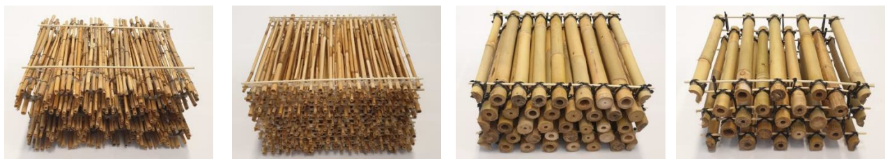
Figure 1. a: Inhomogeneous spacing small scale; b: staggered small scale; c: staggered large scale, high density; d: staggered large scale, low density.
